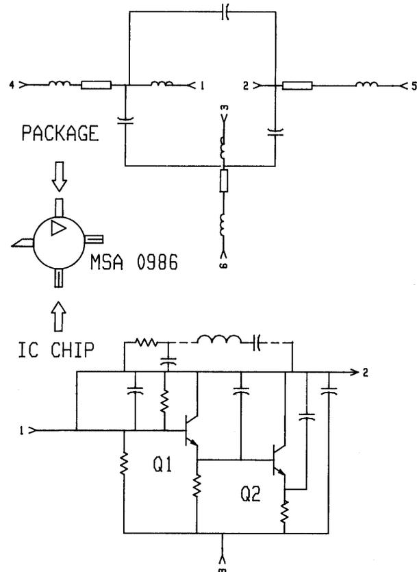
Figure 2. The amplifier model includes both the IC chip equivalent circuit as well as that of the parasitics of the package in which it is embedded.
