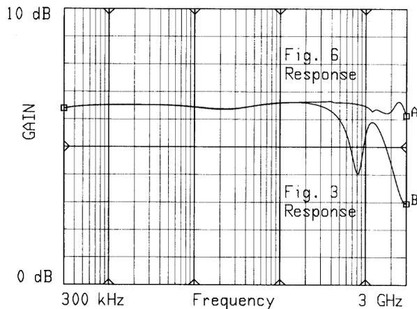
**Figure 7.** Amplifier response with the improvements of Figure 6.
