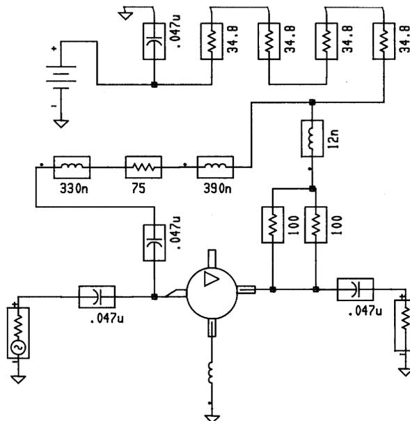
**Figure 3. Complete amplifier with surface mount parts for feedback and bias.**
