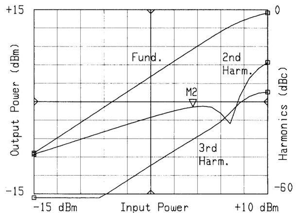
**Figure 8.** Simulated output power (in dBm) and harmonics (in dBc) versus input power (in dBm) at 2 GHz.
