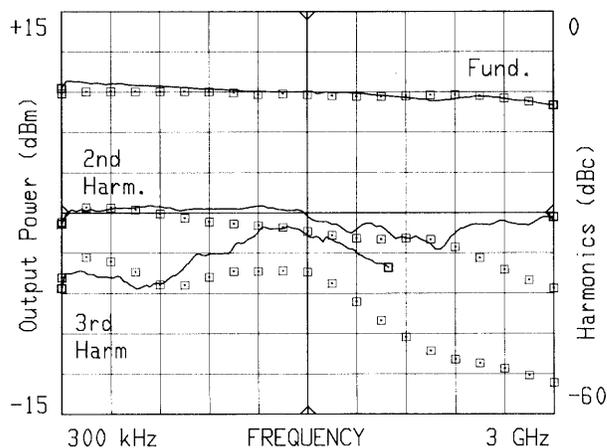
**Figure 11.** Measured (shown as solid line) and simulated (shown as boxes) power and harmonics versus frequency.
