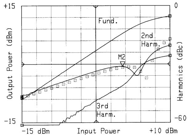
**Figure 10.** Measured power and harmonics for an IC amplifier (shown as solid line) and simulated second harmonics shown as boxes, at 2 GHz.
