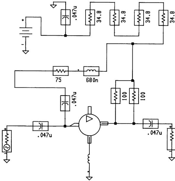
**Figure 6.** The circuit has a modified feedback network using two smaller inductors and an RF choke in the bias to improve high-end response.
