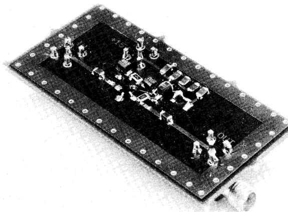
**Figure 12. Photograph of a nearly complete surface mount amplifier circuit that is used for testing power-compression properties.**
