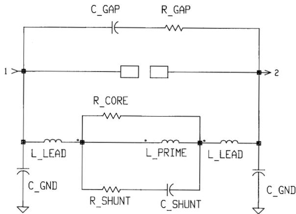
**Figure 4.** This complex circuit is used to model a library of surface-mount inductors of various values. Selecting the appropriate value (label) from the library evokes the respective parasitics for that part.
