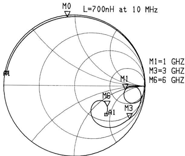
**Figure 5.** This Smith chart plot depicts the measurement of a 680 nH surface-mount inductor. Notice that it resonates near 270 MHz, 1 GHz and 6 GHz.
