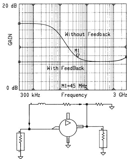
Figure 1. Response of the example IC amplifier in an ideal circuit with and without feedback to control low-end gain.
